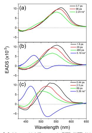
Fig. 6 Evolution-associated difference spectra (EADS) of HPTS obtained from transient absorption results in (a)  $\omega = 1$ , (b)  $\omega = 15$  water-in-oil RMs, and (c) bulk water. The fastest components represent the solvation dynamics; the next two are the proton transfer dynamics. The slowest components shown in  $\omega$  = 15 RMs and bulk water represent the deprotonated species of HPTS (population dynamics)
