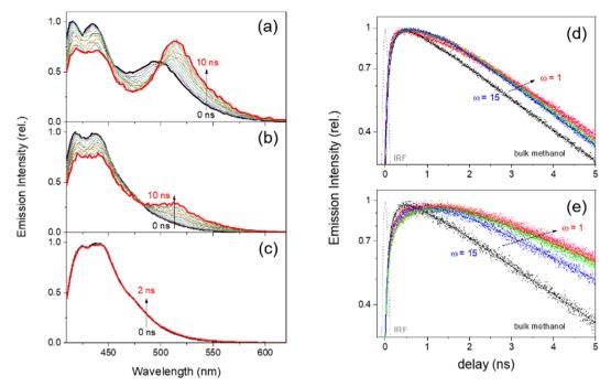
Fig. 4 Time-resolved area-normalized emission spectra (TRANES) of HPTS in *methanol-in-oil* Igepal RMs of (a)  $\omega=1$  and (b)  $\omega=8$ , and (c) bulk methanol; emission kinetics of HPTS in *methanol-in-oil* RMs probed at (d) 440 (neutral) and (e) 510 nm (deprotonated). The 405 nm excitation was used for all the emission measurements, and the instrumental response function (IRF) of the fluorescence measurements was also displayed.
