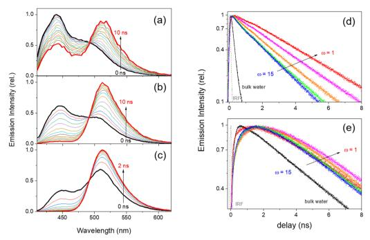
Fig. 3 Time-resolved area-normalized emission spectra (TRANES) of HPTS in water-in-oil Igepal RMs of (a)  $\omega = 1$  and (b)  $\omega = 15$ , and (c) bulk water; emission kinetics of HPTS in water-in-oil RMs probed at (d) 440 (neutral) and (e) 510 nm (deprotonated). The 405 nm excitation was used for all the emission measurements, and the instrumental response function (IRF) of the fluorescence measurements was also displayed
