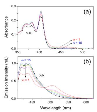
Fig. 2 (a) Steady-state absorption and (b) emission spectra of HPTS in bulk methanol and *methanol-in-oil* Igepal RMs of  $\omega=1$ , 3, 5, 8, and 15. Absorption and emission spectra of HPTS obtained in bulk methanol were displayed as dotted lines for comparison. The emission spectra were normalized with respect to the absorbance of each sample at the excitation wavelength of 405 nm.
