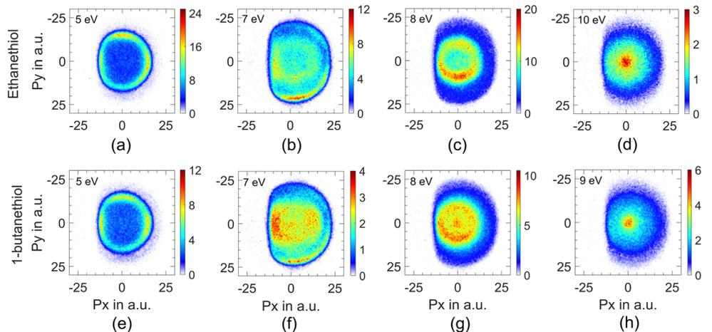
Fig. 2 Momentum images for the  $\text{H}^-$  ions at (a) 5 eV, (b) 7 eV, (c) 8 eV and (d) 10 eV from ethanethiol and (e) 5 eV, (f) 7 eV, (g) 8 eV and (h) 9 eV electron energy from 1-butanethiol. The direction of the electron beam is from top to bottom.
