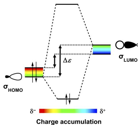
**Fig. 4** A larger accumulation of negative charge ( $\delta^-$ ) destabilizes the occupied molecular orbitals ( $\sigma_{HOMO}$ ) of H-bond acceptors, while a larger accumulation of positive charge ( $\delta^+$ ) stabilizes the unoccupied molecular orbitals ( $\sigma_{LUMO}$ ) of H-bond donors. This results in a smaller HOMO–LUMO energy gap ( $\Delta\epsilon$ ) and therefore a better  $\sigma$ -orbital interaction in case of enhanced charge accumulation.
