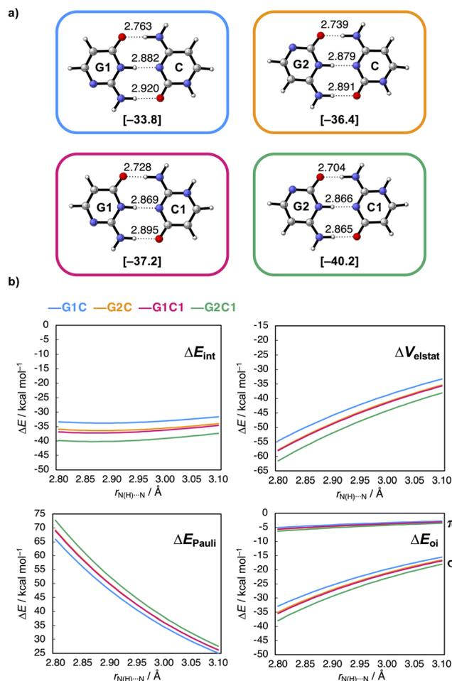
**Fig. 2** (a) Hydrogen-bonded GC base-pair isosteres with equilibrium hydrogen-bond distances (in Å) and interaction energy  $\Delta E_{\text{int}}$  (in kcal mol<sup>-1</sup> in between brackets) and (b) decomposed interaction energy terms ( $\Delta E_{\text{int}} = \Delta V_{\text{elstat}} + \Delta E_{\text{Pauli}} + \Delta E_{\text{oi}} (+ \Delta E_{\text{disp}})$ ) as a function of the middle H-bond distance  $r_{\text{N(H)}\cdots\text{N}}$  (in Å, step size of 0.01 Å).
