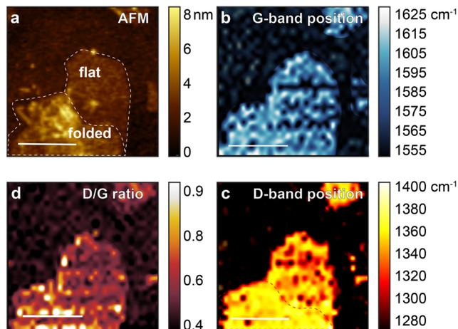
Fig. 2 (a) AFM image of rGO1 (reduced for seven days) on a gold surface, showing a large flake with wrinkles and folded region on the bottom left on the image. TERS map of rGO1, showing (b) the distribution of the G-band position, close to  $1600\text{ cm}^{-1}$  Raman shift. (c) D-Band peak position shift, at close to  $1350\text{ cm}^{-1}$ , and (d) the area ratio of D-band and G-band modes,  $I_D/I_G$ . Scale bar  $1\text{ }\mu\text{m}$ .
