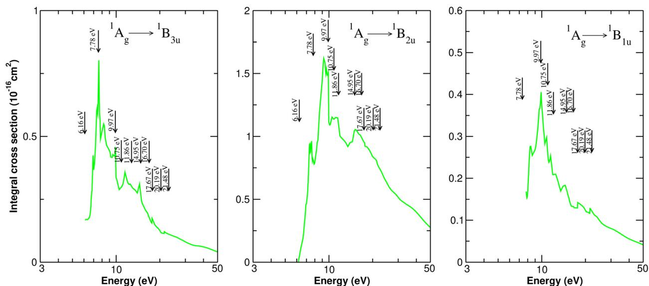
Fig. 8 Integral cross sections for the excitation from the ground state to the  ${}^1B_{3u}$  (5.39 eV),  ${}^1B_{2u}$  (6.16 eV) and  ${}^1B_{1u}$  (7.28 eV) excited states of pyrazine by electron impact. Solid green line, present SMCPP results.
