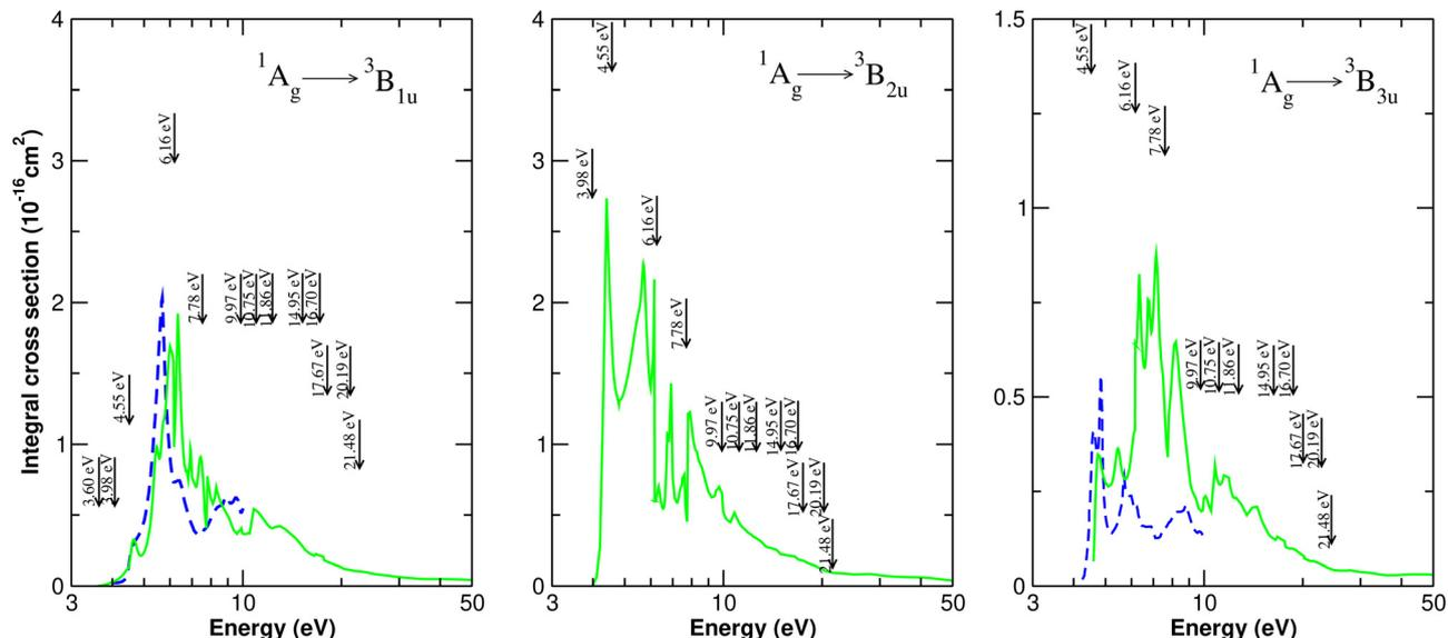
Fig. 7 Integral cross sections for the excitation from the ground state to the  ${}^3B_{1u}$  (3.60 eV),  ${}^3B_{2u}$  (3.98 eV) and  ${}^3B_{3u}$  (4.55 eV) excited states of pyrazine by electron impact. Solid green line, present SMCPP results; dashed blue line, R-matrix results from Mašin and Gorfinkiel.<sup>6</sup>
