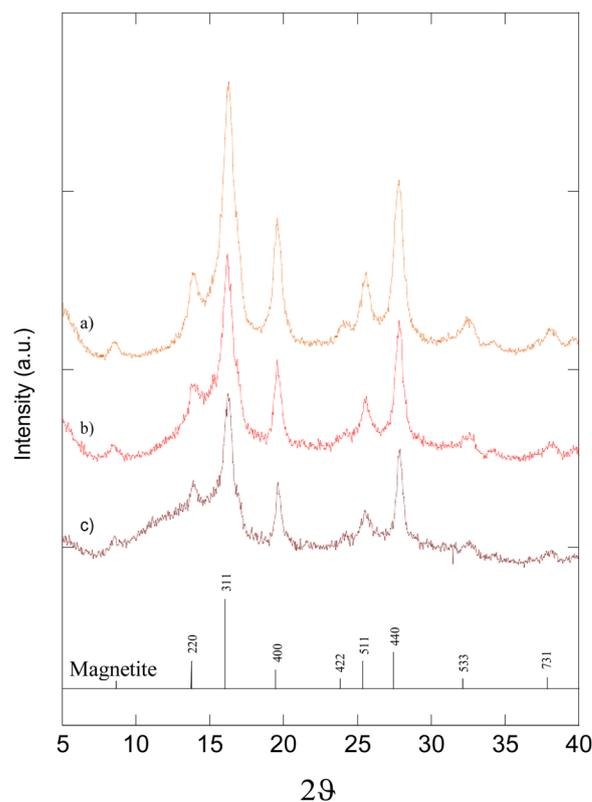
Fig. 1 XRPD patterns of the Fe<sub>3</sub>O<sub>4</sub>/SiO<sub>2</sub> nanocomposites: (a) 6-Fe<sub>3</sub>O<sub>4</sub>/SiO<sub>2</sub> with 6.0 wt% of SiO<sub>2</sub>, (b) 20-Fe<sub>3</sub>O<sub>4</sub>/SiO<sub>2</sub> with 20.0 wt% of SiO<sub>2</sub>, and (c) 50-Fe<sub>3</sub>O<sub>4</sub>/SiO<sub>2</sub> with 50.0 wt% of SiO<sub>2</sub>, respectively.
