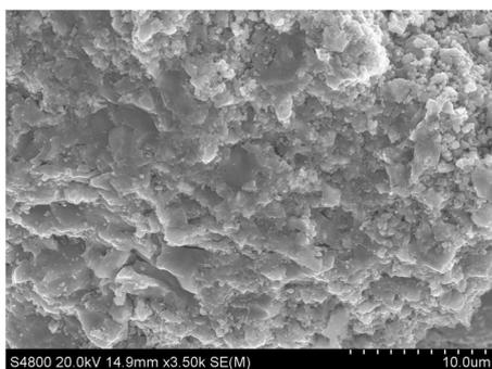
Fig. 3 SEM micrograph of 6- $\text{Fe}_3\text{O}_4/\text{SiO}_2$  nanocomposite.
