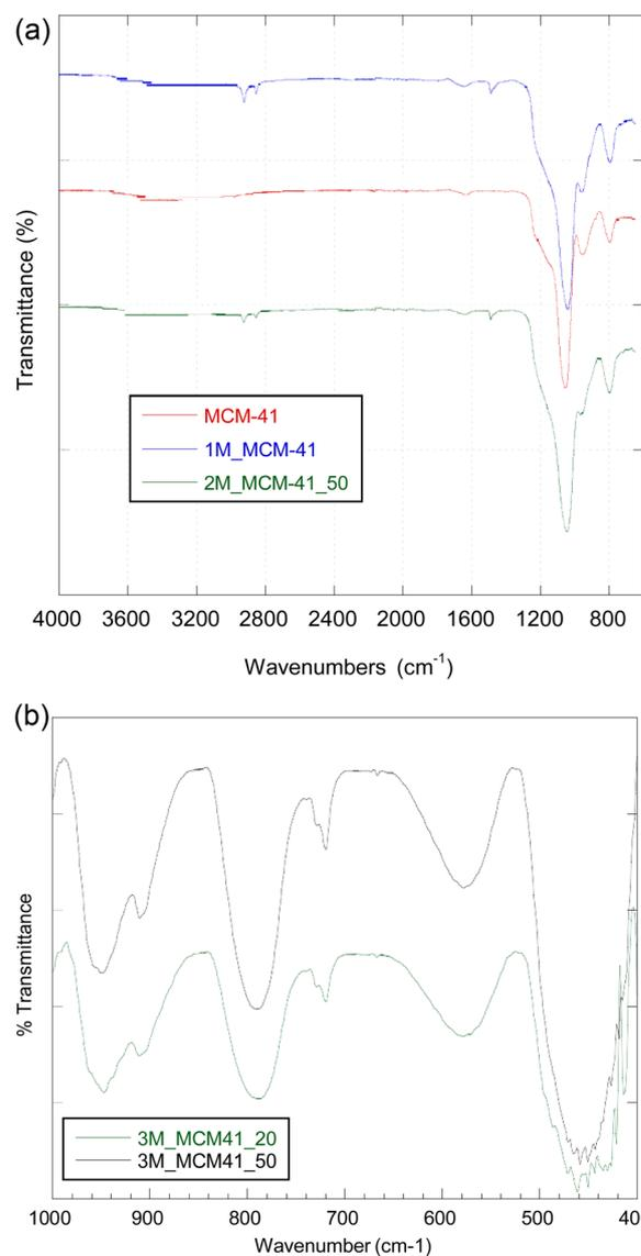
Fig. 13 (a) FTIR spectra of the MCM41 and M\_MCM41 samples. (b) FTIR finger print detail of 2M\_MCM41\_20 and 2M\_MCM41\_50 samples.
