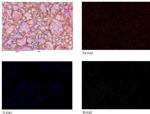
Fig. 4 Left up-side: total elemental distribution map of 6- $\text{Fe}_3\text{O}_4/\text{SiO}_2$  (red spots: iron, green spots: silicon, blue spots: oxygen); right up-side: iron distribution map; left bottom-side: oxygen distribution map; right bottom-side: silicium distribution map.
