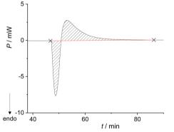
Fig. 2 Thermogram for the formation of BZP-DPA cocrystals (n(BZP) =n(DPA) = 0.165 mmol) performed in the Setaram Calvet calorimeter at 25 °C.
