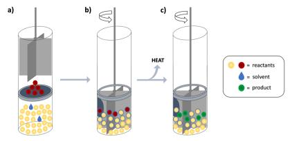
Scheme 1 Calorimetric cell system used and experimental procedure for direct monitoring of reactions in the solid state: (a) equilibration phase; (b) reaction initiation; (c) reaction advancement and heat-flow measurement. A reference cell with a practically identical stirrer, filled with only one reactant is also present in the calorimeter and differential heat power is measured during the experiment.
