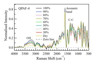
Fig. 13 Normalised Raman spectra from the centre of the QPAF-4 membrane at RH values 30-100% in steps of 10%. The spectra were normalised using the area under the aromatic band. A  $\times 50$  objective lens,  $100~\mu m$  hole, and D1 filter were used during the measurements.
