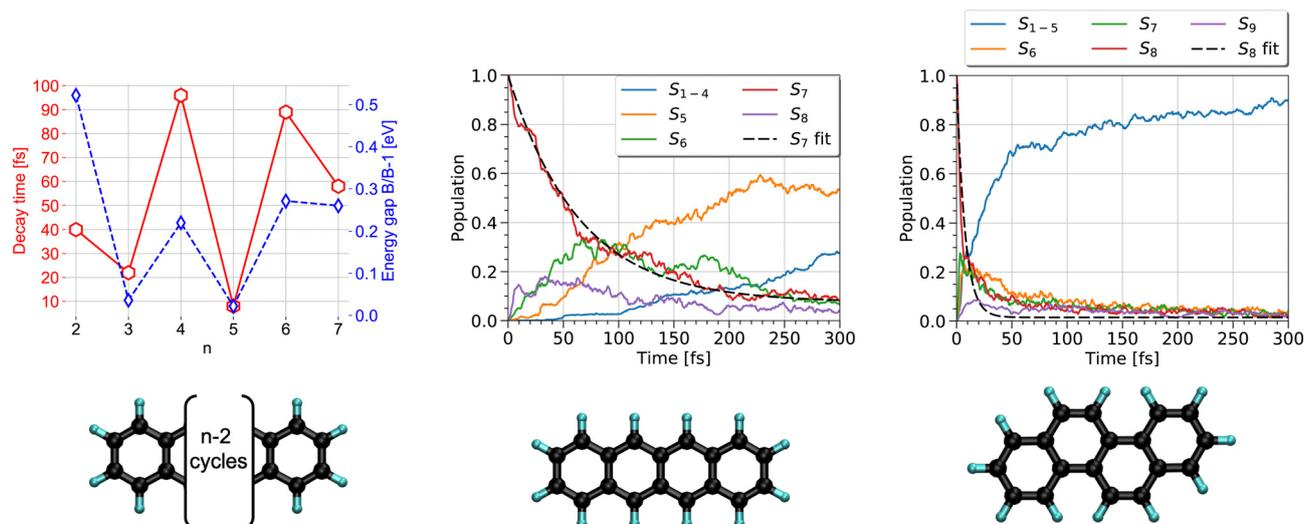
Fig. 5 Left: Correlation between the electronic relaxation timescales from the brightest state and energy gap between the latter and the state just below for polyacenes ( $n$  is the number of aromatic cycles). Time evolution of the state's population for tetracene (middle) and chrysene (right) molecules. Left: Adapted from ref. 191 with permission from the PCCP Owner Societies. Right: Adapted from ref. 216 with acknowledgements of AIP. Copyright 2020.
