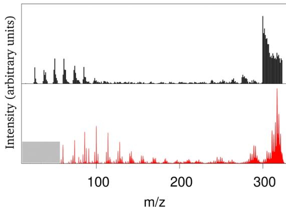
Fig. 2 Experimental (black) and calculated (red) mass spectrum in arbitrary units for coronene heated by successive hydrogenations ( $m/z = 300$ : bare coronene;  $m/z > 300$ : hydrogenated coronene;  $m/z$  between 275 and 285: loss of  $C_2H_n$  fragments). Adapted from ref. 201 with permission from the PCCP Owner Societies. Copyright 2018.
