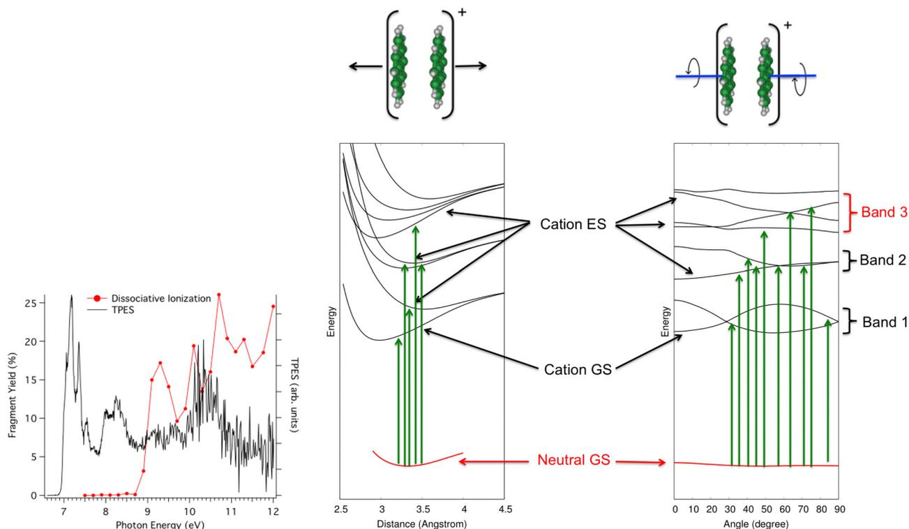
Fig. 8 Left: photoionization (black) and photoionization + dissociation (red) spectra for  $\text{Py}_2$  recorded at SOLEIL synchrotron apparatus. Right: computed electronic ground states of  $\text{Py}_2$  and  $\text{Py}_2^+$  and first electronic excited states of  $\text{Py}_2^+$  according to dissociative breathing mode (left) and non-dissociative twist mode (right). Adapted from ref. 222 with permission from the PCCP Owner Societies. Copyright 2023.
