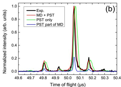
Fig. 4 TOF mass spectra for fragment monomers resulting from proton collision-induced dissociation of the cationic pyrene dimer, measured experimentally or simulated assuming a statistical (PST only) vs. non-statistical dissociation (DFTB-BOMD + PST). Adapted from ref. 213. with permission from Springer Nature. Copyright 2021.
