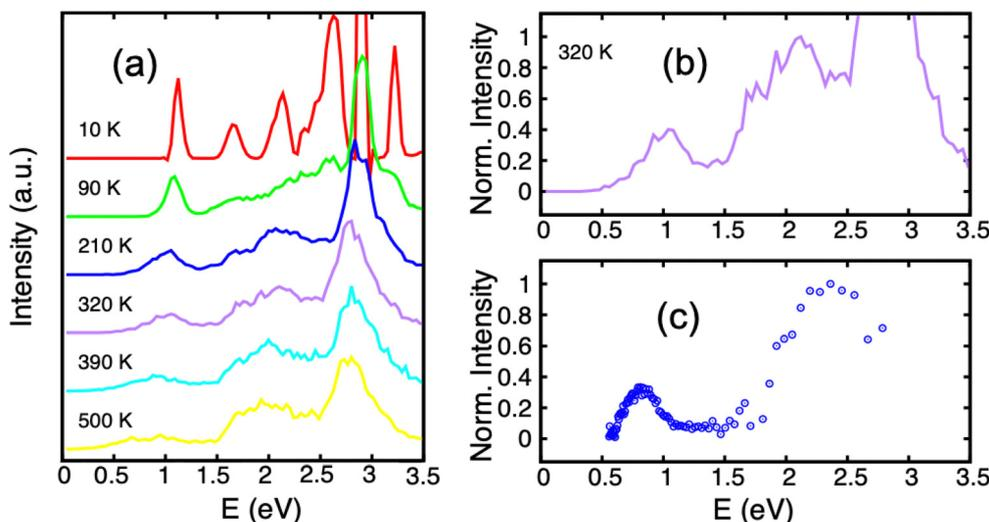
Fig. 7 Experimental action spectrum (photodissociation-c) of  $\text{Py}_2^+$  compared with photoabsorption spectra computed for various temperatures (a) and (b), (DFTB-EXCI). Adapted from ref. 221 with permission from the PCCP Owner Societies. Copyright 2021.
