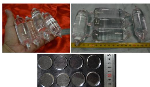
**Enabling cryogenic gravitational wave detectors: growth of sapphire crystals with record low absorption in the near infrared**
