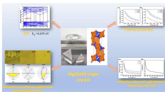
Crystal growth, dislocation, thermodynamic and optical properties, and electronic structure of  $\text{Mg}_2\text{SiO}_4$  single crystals
