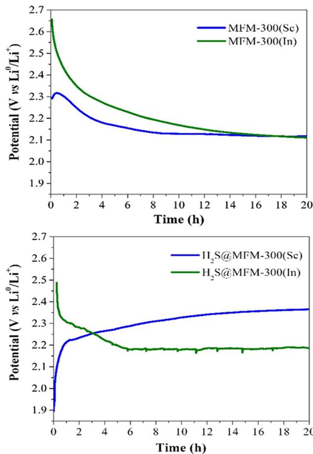
**Fig. 6** Open-circuit potential (OCP) monitoring of MFM-300(M) as active materials in cathodes for lithium-ion batteries to describe the cell stabilisation processes. (Top) Pristine materials MFM-300(Sc) and MFM-300(In); (bottom) H<sub>2</sub>S saturated materials H<sub>2</sub>S@MFM300(Sc) and H<sub>2</sub>S@MFM-300(In). Reproduced with permission from ref. 38. Copyright 2020, American Chemical Society.
