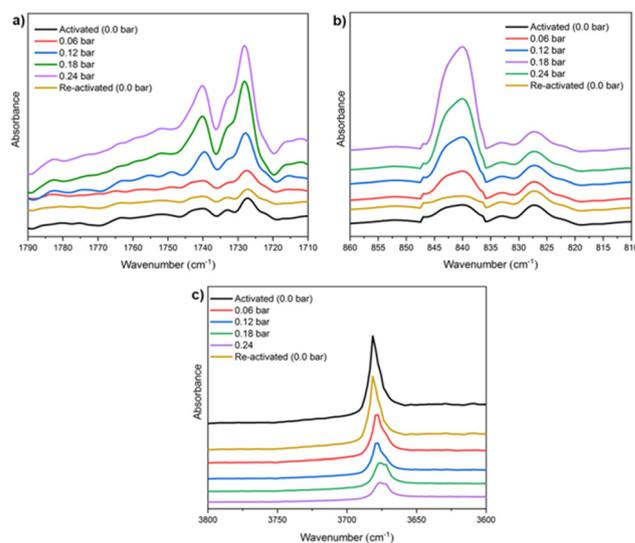
**Fig. 4** DRIFT spectra of  $\text{NH}_3$  adsorbed at different pressures (from 0 to 0.24 bar) over activated MFM-300(Sc) at 298 K, split into three wavenumber regions: (a) 1790–1710  $\text{cm}^{-1}$ ; (b) 860–810  $\text{cm}^{-1}$ ; and (c) 3800–3600  $\text{cm}^{-1}$ . Reproduced with permission from ref. 26. Copyright 2021, American Chemical Society.
