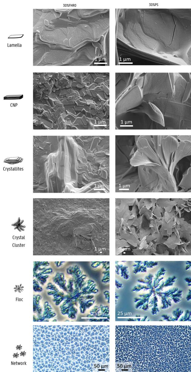
**Fig. 3** Multiscale structure analysis of stearic- and palmitic-based fat blends (30% FHRO and 30% PS in HOSO) visualized through cryo-SEM highlighting lamellar structures, crystalline nanoplatelets (CNPs), CNP aggregates and crystal clusters, and phase contrast microscopy showing floc morphology and aggregation. The iconography to the left is based on Penagos, *et al.*<sup>8</sup>
