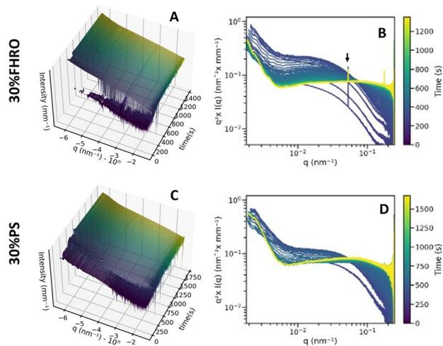
**Fig. 6** USAXS results. In panels A and B, results for a 30% FHRO dilution in HOSO. In panels C and D, USAXS results for a 30% dilution of PS in HOSO. In A and C, surface plots are shown. Panels B and D present a Kratky representation of the data, removing the scattering profiles where only the oil is visible. The data is presented as  $q^2 I$  vs.  $q$ . The arrow presented in panel B corresponds to a hot pixel, hence, this feature does not represent the sample's behavior.
