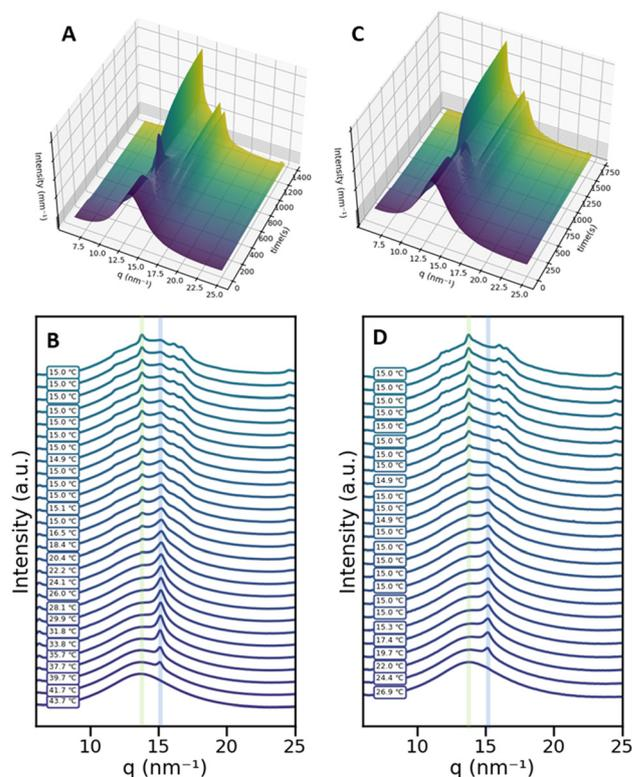
**Fig. 4** WAXS results. In panels A and C, surface plots of the WAXS profiles. In panels B and D, the orthogonal projection of the data expanding on the polymorphic transition. A vertical shift is performed to allow better visualization of each profile. Labels to the left indicate temperature. In panels A and B, a dilution of 30% FHRO in HOSO is presented. In panels C and D, a 30% dilution of PS in HOSO is shown.
