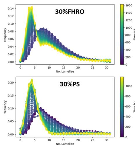
**Fig. 8** Crystallite thickness distributions for a 30% FHRO dilution in HOSO and a 30% PS dilution in HOSO.
