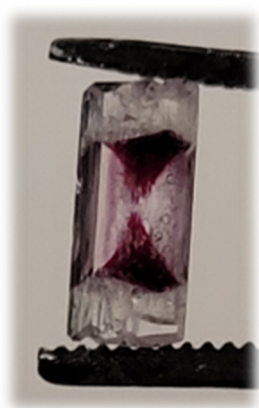
Fig. 7 K_2SO_4 -AF crystal isolated in two successive growth steps: the initial crystal is grown from solutions containing 0.3% AF, generating the hourglass-like AF inclusion; build-up of the pure lattice layer is obtained after 48 hours aging in a supersaturated solution containing no AF.
