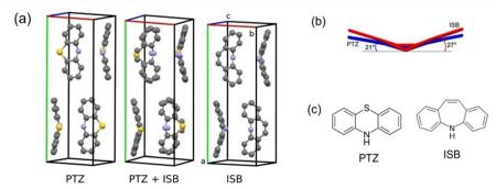
Fig. 1 a) Packing of PTZ and ISB molecules in their lattices and their mixed 1/2 structure PTZ/ISB. The cell orientation has been upright, as it is on the substrate surface. b) The projection of PTZ and ISB molecular structures to illustrate the similarity of the molecular geometry and the bending angles. PTZ is displayed in blue and ISB is in red. c) Molecular structure of PTZ and ISB.
