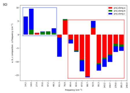
Fig. 7 a) Unit cell of the pristine PTZ (black) superimposed to the PTZ@ISBcell (orange); (b) graphic representation of the result of the dot product between the vibrational eigenvectors of the two structures (purple = 0, yellow = 1). c) Frequency shifts for the modes computed in the 14–240 cm<sup>-1</sup> spectral window, where the mode eigenvectors are decomposed by projection along the crystal axes of the PTZ@ISB system.
