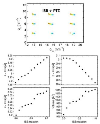
Fig. 3 Summary of grazing incidence X-ray diffraction peak positions of various fractions of ISB:PTZ measured on spin coated samples. The extracted cell dimensions of the various samples hosting different amounts of PT7 and ISB
