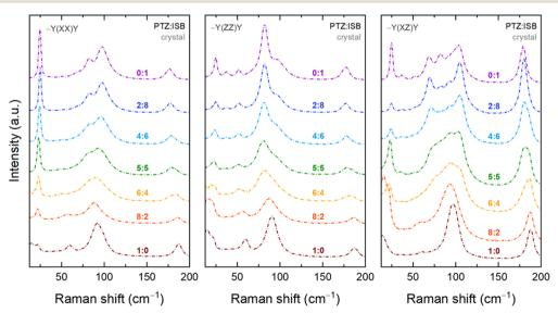
Fig. 5 Polarized lattice-phonon Raman spectra of PTZ:ISB solid solutions at given molar ratios in crystal samples: labels Y(XX)Y and Y(ZZ)Y identify an experimental configuration in which modes of  $A_g$  symmetry are detected; label Y(XZ)Y identifies an experimental configuration in which modes of  $B_{2\alpha}$  symmetry are detected.
