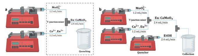
Fig. 2 Schematic representation of the (a) first and (b) second microfluidic setup. The dashed line indicates the portion of the setup immersed in a cold bath at -4 °C.
