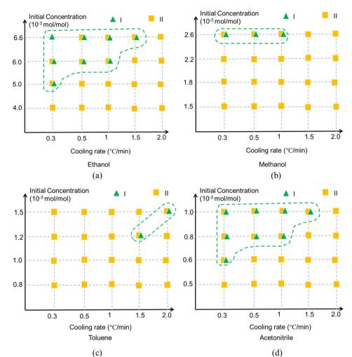
Fig. 12 Crystallisation outcomes of TFA as a function of cooling rate and initial concentration in (a) ethanol, (b) methanol, (c) toluene and (d) acetonitrile. Green triangle represents form I while yellow square represents form II. The overlapping patterns represent that the results are stochastic since form I and form II both have probability to crystallise at the same conditions. The areas highlighted indicate the crystallisation environments favoured by form I.
