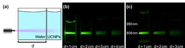
Fig. 5 (a) Schematic diagram of excitation of surface modified UCNP by an 808 nm laser penetrating water. (b) The digital photos of UCL of CSSS NPs excited by the 808 nm laser after passing through 1–4 cm water. (c) The digital photos of UCL of surface modified CSSS NPs dispersed in deionized water excited by 980 nm and 808 nm lasers after passing through 1–3 cm water.
