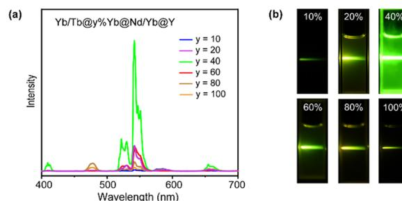
Fig. 3 (a) Upconversion luminescence spectra of  $\text{Tb}/\text{Yb}@ \text{y}\% \text{Yb}@ \text{Nd}/\text{Yb}@ \text{Y}$  ( $y = 10$ – $100$ ) CSSS NPs. (b) Digital photos of  $\text{Tb}/\text{Yb}@ \text{y}\% \text{Yb}@ \text{Nd}/\text{Yb}@ \text{Y}$  ( $y = 10$ – $100$ ) CSSS NPs.
