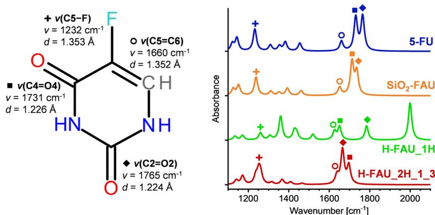
Fig. 4 Left: 5-FU molecule including bond distances and stretching frequencies of the four most prominent modes in the wavenumber range from 1200 to 1800  $\text{cm}^{-1}$ . Right: DFT-calculated IR spectra of free 5-FU (top curve) and adsorbed 5-FU. Spectra are normalised to have the same maximal intensity in the shown wavenumber range.
