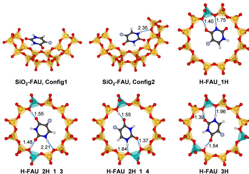
Fig. 3 Lowest-energy configurations of 5-FU in FAU. For SiO<sub>2</sub>-FAU, the surrounding portion of the framework is shown, whereas only the 12MR containing the Al atom(s) is shown for protonic FAU models. Hydrogen bonds are displayed as blue lines, with distances given in Å.
