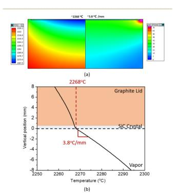
Fig. 3 (a) Temperature distribution and temperature gradient in the PVT reactor near the growth front obtained with FE analysis and (b) vertical temperature distribution along axisymmetric line.
