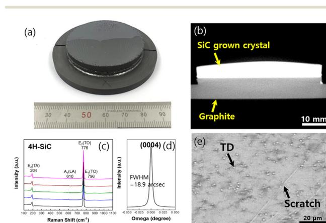
**Fig. 4** (a) The grown SiC crystal (growth rate 1.46 mm h<sup>-1</sup>) and its evaluation results with (b) cross-sectional tomography, (c) micro-Raman spectroscopy, (d) X-ray rocking curve, and (e) X-ray topography.
