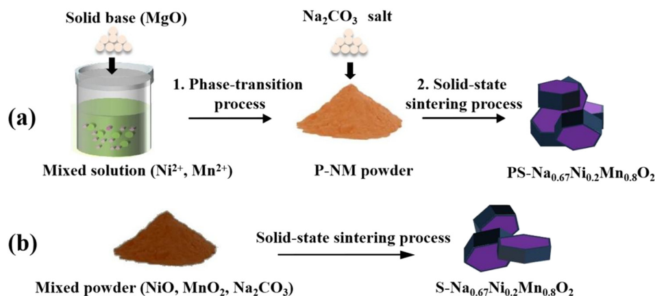
Fig. 1 Schematic illustration for the preparation process of (a) PS- \text{Na}_{0.67}\text{Ni}_{0.2}\text{Mn}_{0.8}\text{O}_2 and (b) S- \text{Na}_{0.67}\text{Ni}_{0.2}\text{Mn}_{0.8}\text{O}_2 .
