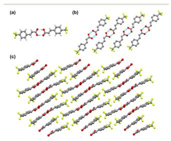
Fig. 3 Crystal structure of 4-tfmca: (a) asymmetric unit, (b) onedimensional string of dimers along the b axis, and (c) layered structure composed of the one-dimensional layers along the b axis. For b and c, hydrogen atoms are not displayed for clarity reasons.
