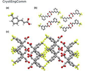
Fig. 4 Crystal structure of 3-tfmca: (a) asymmetric unit, (b) two dimer orientations that are almost perpendicular to each other, and (c) zigzag structure. For b and c, the hydrogen atoms are not displayed for clarity reasons.
