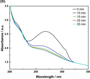
Fig. 8 FTIR and UV spectra of 4-tfmca in KBr pellets as a function of irradiation time: (a) FTIR spectra and (b) UV spectra.
