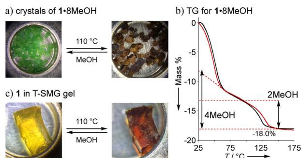
**Fig. 5** a) The appearances and b) TG studies of the reversible guest insertion-release processes for 1·8MeOH: TGA shows 7MeOH; the scanning rate of 5 °C min<sup>-1</sup>. c) Reversible color change of the T-SMG gel with **1** by MeOH.
