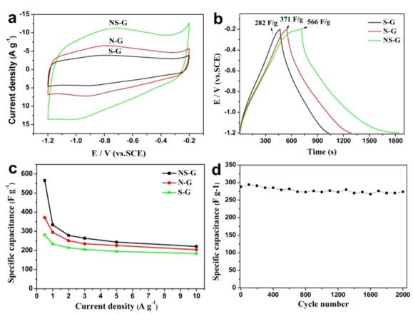
Fig. 3 (a) CVs measured at 30 mV s<sup>-1</sup> and (b) GCD curves measured at 0.5 A g<sup>-1</sup> of NS-G, N-G and S-G samples. (c) The specific capacitance of NS-G, N-G and S-G at different current densities and (d) cycle performance of NS-G at a current density of 3.0 A g<sup>-1.24</sup> 2015 Springer Nature, published under a CC license (open access).
