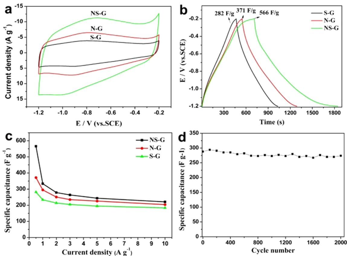
Fig. 3 (a) CVs measured at  $30 \text{ mV s}^{-1}$  and (b) GCD curves measured at  $0.5 \text{ A g}^{-1}$  of NS-G, N-G and S-G samples. (c) The specific capacitance of NS-G, N-G and S-G at different current densities and (d) cycle performance of NS-G at a current density of  $3.0 \text{ A g}^{-1}$ .<sup>24</sup> 2015 Springer Nature, published under a CC license (open access).
