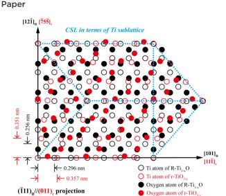
Fig. 12 Schematic drawing of the  $(\bar{1}11)_R//(011)_r$  interface in top view with Ti (open circle) and O (solid circle) atoms denoted in black and red for R and r, respectively with CSL in terms of the periodic match of Ti atoms outlined by blue dashed lines.
