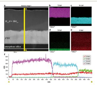
Fig. 3 Compiled STEM results of the titanium oxide thin film as deposited on FTO-coated silica glass by the PLA process under 600 mJ per pulse in vacuum: (a) HAADF image; (b)-(e) EDX mapping and (f) EDX line scan from position A to B in (a), showing Ti inward and Sn outward diffusion in a narrow (ca. 50 nm thick) interdiffusion zone.
