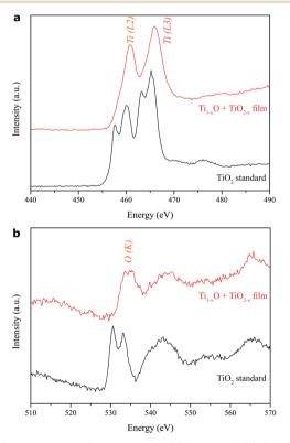
Fig. 8 Electron energy loss spectra of (a) Ti  $L_{2,3}$  and (b) O K edge of the R-Ti<sub>1-x</sub>O + r-TiO<sub>2-x</sub> predominant thin film as deposited on the FTO-coated silica glass by the PLA process under 600 mJ per pulse in vacuum (red traces) in comparison with the rutile TiO<sub>2</sub> standard (black traces, EELS Atlas, Gatan Inc.).
