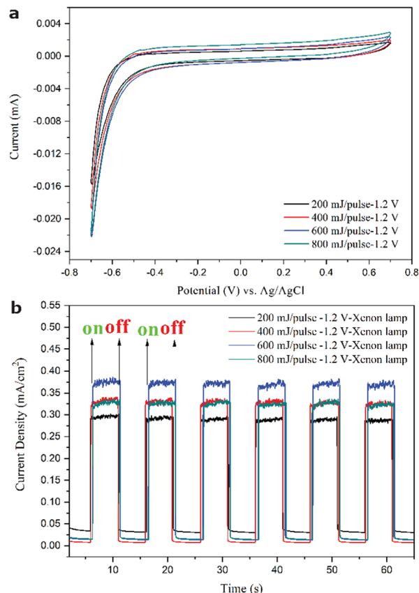
**Fig. 11** Cyclic voltammetry (a) and chopped current density–time curve (b) of a photoelectrochemical cell using the titanium oxide film/FTO as the working electrode in a three-electrode configuration with 1.2 V external bias under xenon illumination, indicating that a sample prepared with the optimum pulse energy (*i.e.* 600 mJ per pulse) has the highest current density.
