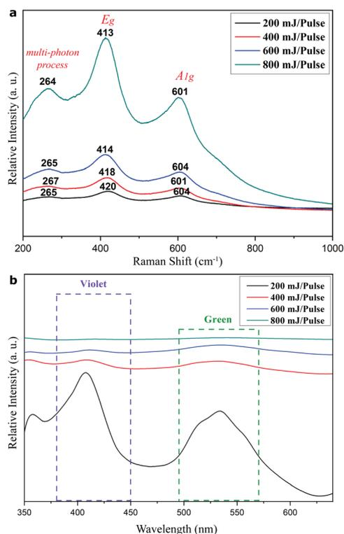
Fig. 9 (a) Raman and (b) PL spectra of the  $\text{R-Ti}_{1-x}\text{O} + \text{r-TiO}_{2-x}$  predominant thin film as deposited on the FTO-coated silica glass by the PLA process in vacuum under specified laser pulse energies of 200, 400, 600 and 800 mJ per pulse, respectively.
