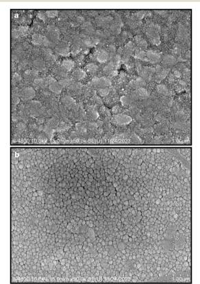
Fig. 2 Top-view SEM SEI of the titanium oxide thin film (a) as deposited on FTO-coated silica glass under 200 mJ per pulse for 30 min in vacuum and (b) after annealing at 450 °C for 5 h in air.
