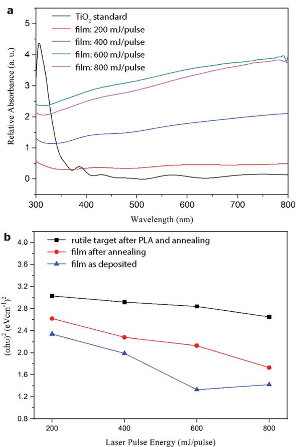
Fig. 10 (a) UV-vis absorbance spectra and (b) the corresponding band gap of the  $\text{R-Ti}_{1-x}\text{O} + \text{r-TiO}_{2-x}$  predominant thin film as deposited on the FTO-coated silica glass by the PLA process in vacuum under 200, 400, 600 and 800 mJ per pulse, respectively, vs. that subject to further annealing at 450 °C in air for 5 h. The control group is the ablated  $\text{TiO}_2$  rutile target without/with further 450 °C annealing in air for 5 h.
