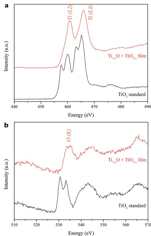
**Fig. 8** Electron energy loss spectra of (a) Ti  $L_{2,3}$  and (b) O K edge of the r- $Ti_{1-x}O$  + r- $TiO_{2-x}$  predominant thin film as deposited on the FTO-coated silica glass by the PLA process under 600 mJ per pulse in vacuum (red traces) in comparison with the rutile  $TiO_2$  standard (black traces, EELS Atlas, Gatan Inc.).
