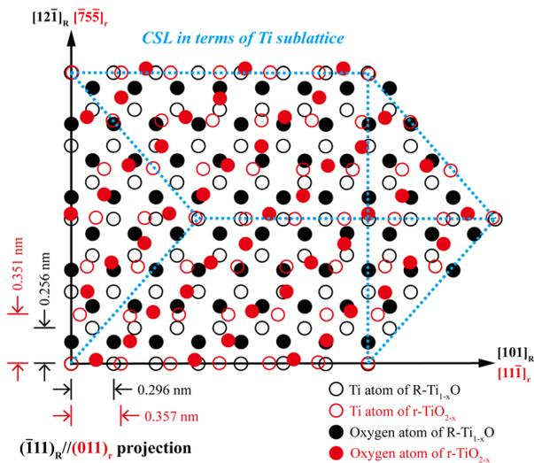
**Fig. 12** Schematic drawing of the  $(\bar{1}\bar{1}\bar{1})_R/(011)_r$  interface in top view with Ti (open circle) and O (solid circle) atoms denoted in black and red for R and r, respectively with CSL in terms of the periodic match of Ti atoms outlined by blue dashed lines.
