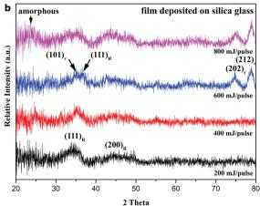
Fig. 1 XRD traces of titanium oxide thin films as deposited on the substrates of (a) FTO-coated silica glass and (b) silica glass by the PLA process for 30 min in vacuum under 200, 400, 600, and 800 mJ per pulse, respectively. Note that  $R-Ti_{1-x}O$  and  $r-TiO_{2-x}$  condensates are not concentrated enough in the film to show appreciable diffraction, in contrast with the overwhelming signals of cassiterite polycrystals from the FTO underneath in (a).
