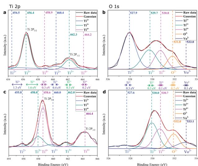
**Fig. 7** Ti 2p (left panel) and O 1s (right panel) XPS spectra of the titanium oxide thin film as deposited on the FTO-coated silica glass by the PLA process in vacuum under specified pulse energies of (a and b) 600 mJ per pulse and (c and d) 800 mJ per pulse.
