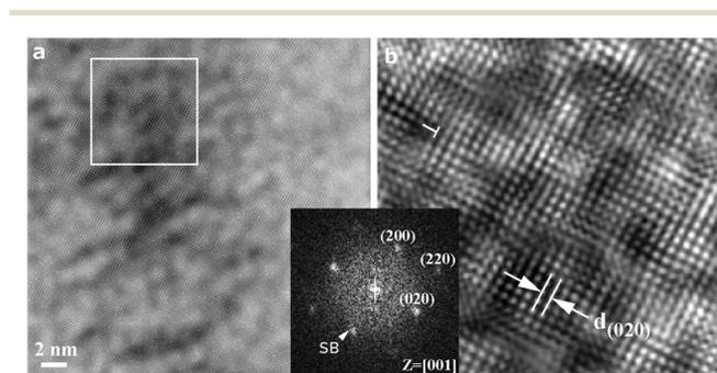
**Fig. 5** TEM (a) lattice image of the R-Ti<sub>1-x</sub>O rich domain and (b) magnified square region with FFT (inset) showing dislocation ( $\perp$ ) and paracrystalline distribution of defect clusters with an interspacing *ca.* 5 times (020) lattice fringes corresponding to sideband (SB) diffractions in the [001]<sub>R</sub> zone axis. FIB sample from a film deposited on the FTO-coated silica glass under 200 mJ per pulse.
