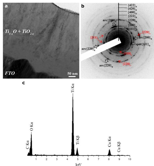
Fig. 4 TEM images of (a) BFI coupled with (b) SAED pattern and (c) EDX spectrum of the titania oxide thin film (predominantly R- $\text{Ti}_{1-x}\text{O}$  with preferred orientation and minor r- $\text{TiO}_{2-x}$ ) as deposited on FTO-coated silica glass by the PLA process under 600 mJ per pulse in vacuum.
