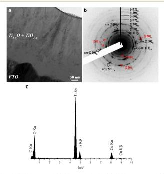
Fig. 4 TEM images of (a) BFI coupled with (b) SAED pattern and (c) EDX spectrum of the titania oxide thin film (predominantly R-Ti<sub>1-x</sub>O with preferred orientation and minor r-TiO<sub>2-x</sub>) as deposited on FTOcoated silica glass by the PLA process under 600 mJ per pulse in vacuum.
