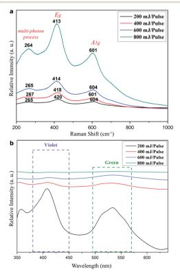
Fig. 9 (a) Raman and (b) PL spectra of the  $R-Ti_{1-x}O$  +  $r-TiO_{2-x}$ predominant thin film as deposited on the FTO-coated silica glass by the PLA process in vacuum under specified laser pulse energies of 200, 400, 600 and 800 mJ per pulse, respectively.
