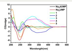
Fig. 4 The CD spectra of Na<sub>2</sub>dUMP, Na<sub>2</sub>UMP, and 1-5 in solid state (KCl:[sample] = 200:1).
