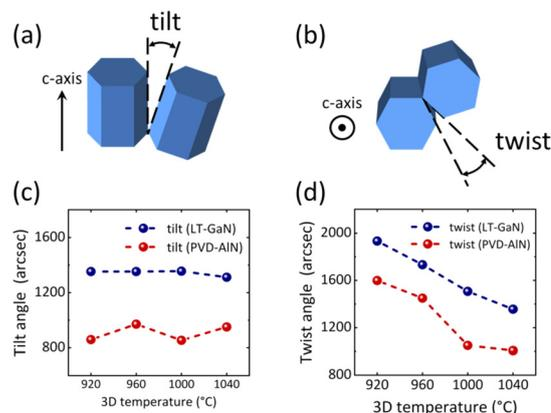
**Fig. 4** Schematic diagram of (a) tilt angle and (b) twist angle between GaN grain columns. (c) Tilt and (d) twist angles of the samples A1–A4 and B1–B4 after 3D growth calculated from the  $\omega$ -scans for symmetrical planes and  $\omega/\varphi$ -scans for asymmetrical planes.
