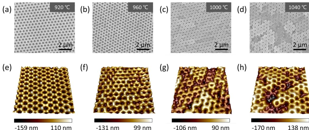
**Fig. 3** Plane-view SEM images of interrupted samples after 3D GaN growth on NPSS using PVD-AlN NLs, corresponding to 3D temperatures of (a) 920 °C, (b) 960 °C, (c) 1000 °C, and (d) 1040 °C. All scale bars denote 2  $\mu\text{m}$ . AFM images of these interrupted samples with 3D temperatures of (e) 920 °C, (f) 960 °C, (g) 1000 °C, and (h) 1040 °C. The AFM images correspond to 5  $\mu\text{m}$  square regions.
