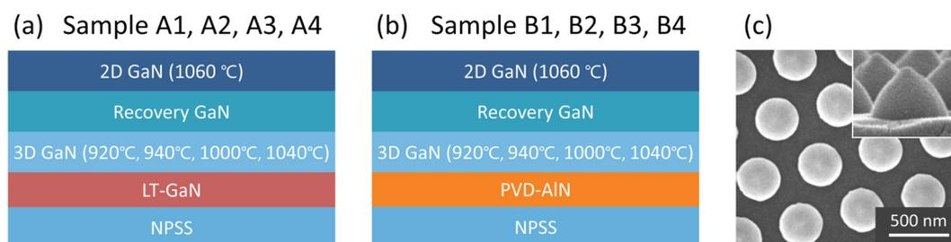
**Fig. 1** Schematic diagrams of GaN films grown on NPSS with (a) *in situ* LT-GaN NLs (samples A1–A4) and (b) *ex situ* PVD-AlN NLs (samples B1–B4). The order from 1 to 4 represents a gradual increase in 3D temperature. (c) A plane-view SEM image of NPSS; the inset shows a cross-sectional SEM image of the NPSS.
