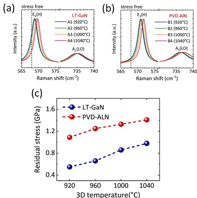
Fig. 9 Raman spectra of GaN films grown on NPSS with (a) LT-GaN NLs and (b) PVD-AlN NLs at different 3D temperatures. (c) The residual compressive stresses calculated from the GaN  $E_2(\text{H})$  phonon peak position.
