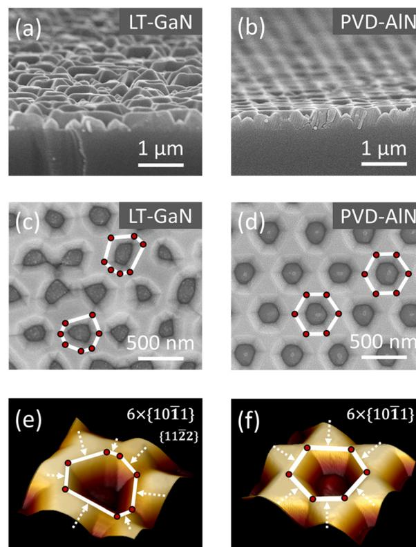
Fig. 5 Cross-sectional SEM images of the interrupted samples of A1 and B1 after 3D growth on NPSS with (a) LT-GaN and (b) PVD-AlN NLs. Plane-view SEM images of these interrupted samples with (c) LT-GaN and (d) PVD-AlN NLs. 3D AFM images of these interrupted samples with (e) LT-GaN and (f) PVD-AlN NLs. The white boxes and red dots depict the GaN sidewall profile, and the white dashed lines with arrows indicate the GaN growth rates along growth directions.
