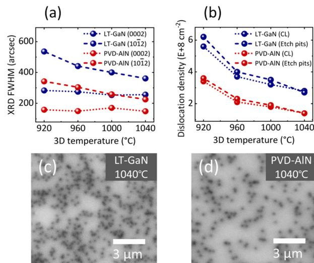
Fig. 7 (a) XRD FWHMs of the (0002) and (10 $\bar{1}2$ ) planes of GaN films. (b) Variation of dislocation densities in GaN films grown on NPSS with different 3D temperatures obtained by CL imaging and counting etch pits by AFM. Plane-view CL mapping of GaN films for (c) sample A4 with LT-GaN NLs and (d) sample B4 with PVD-AlN NLs.
