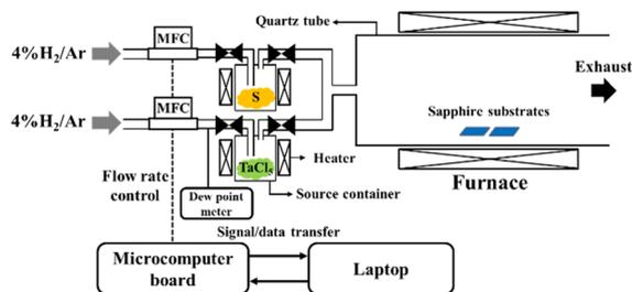
Fig. 1 An APCVD with a separate-flow system for synthesizing epitaxial  $\text{TaS}_2$  films. All the parameters (the flow rates of the sulphur line and  $\text{TaCl}_5$  line, the temperatures of sulphur and  $\text{TaCl}_5$ , and reaction temperature) were separately controlled. MFC represents a mass flow controller.
