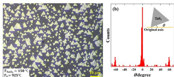
Fig. 4 (a) OM image at the edge of the sapphire to count the isolated triangle domains. (b) Orientation histogram of TaS<sub>2</sub> thin films showing the unidirectional growth. The inset shows the geometrical relationship between the original axis and measured theta ( $\theta$ ).
