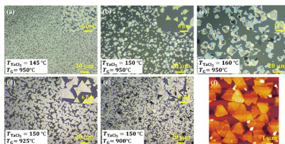
**Fig. 3** (a)–(e) OM images of epitaxially grown TaS<sub>2</sub> films at various TaCl<sub>5</sub> temperatures ( $T_{\text{TaCl}_5}$ ) and growth temperatures ( $T_G$ ) (sample numbers (i)–(v)). The enlarged images at the centres of the individual ones are shown as insets to observe the shape of the domains. (f) Magnified AFM image of sample (a).
