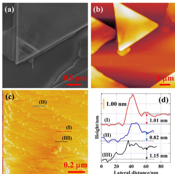
**Fig. 8** (a) SEM image of the TaS<sub>2</sub> triangle domain. This is a magnified area of the rectangle shown in Fig. S9(a).† (b) AFM image of the TaS<sub>2</sub> triangle domain. (c) Step-and-terrace structure on the surface of the TaS<sub>2</sub> triangle domain shown in Fig. 8(b). (d) Step height profiles at lines (I)–(III) in (c). The average step height was calculated to be 0.99 nm.
