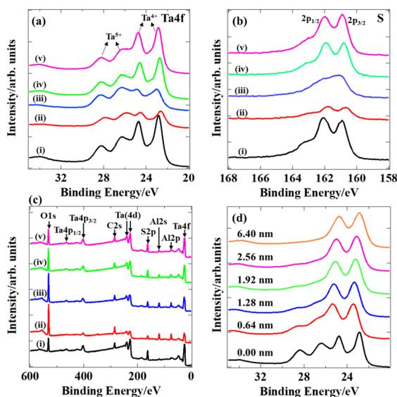
Fig. 7 XPS spectra of the selected elements (a) tantalum (b) and sulphur, and (c) wide scan XPS spectra. Ta<sup>5+</sup> shows surface oxidation due to air exposure. No chlorine was detected, meaning the complete decomposition of TaCl<sub>5</sub>. (d) Depth profile of sample (iv) with unidirectional triangle domains for Ta 4f. The thickness of the native oxide was less than 2.56 nm.
