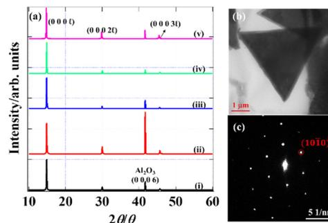
Fig. 5 (a) XRD patterns of samples (i)–(v). Only the diffraction peaks that originated from the basal plane were observed and labelled (0 0 0 *l*), (0 0 0 2 *l*), and (0 0 0 3 *l*). The peaks at around 41.7 degrees originated from the *c*-plane sapphire substrates. The calculated interlayer distance (0.596 ± 0.002 nm) is consistent with the reported values. (b) TEM image of sample (iv). (c) Electron diffraction pattern of the triangle domain shown in (b).
