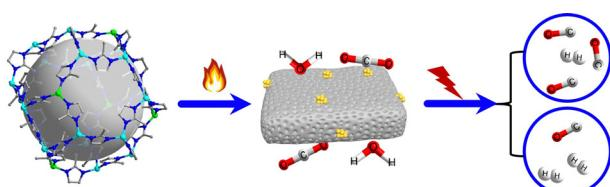
Cu-nanocluster-loaded N-doped porous graphitic carbon for electrochemical CO<sub>2</sub> reduction towards syngas generation
