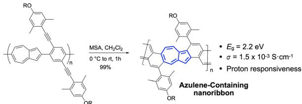
**Synthesis of an azulene-containing graphene nanoribbon**
