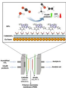
**Surface modified copper foam with cobalt phthalocyanine carbon nanotube hybrids for tuning CO<sub>2</sub> reduction reaction products**
