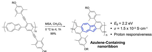
**Synthesis of an azulene-containing graphene nanoribbon**
