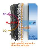
Enhanced CO<sub>2</sub> reduction with hydrophobic cationic-ionomer layer-modified zero-gap MEA in acidic electrolyte
