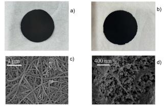
Fig. 13 Photographs of neat SWCNT-BP (a) and bioMOF@SWCNT-BP obtained by integrating Cu<sub>6</sub>SrThreo and SWCNT-BP (b) circular membranes own an average diameter of 41  $\pm$  1 mm. SEM images of SWCNT-BP (c) and bioMOF@SWCNT-BP (d). This figure is reproduced with permission from ref. 78, copyright ACS 2022.
