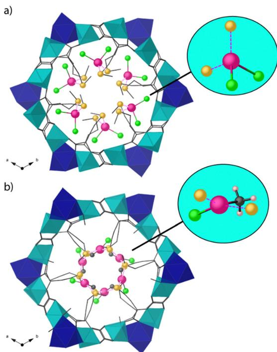
Fig. 6 Perspective views of one single channel of bioMOF **Cu<sub>6</sub>CaMet** after capturing HgCl<sub>2</sub> (a) and CH<sub>3</sub>HgCl (b). Copper and calcium atoms are represented by cyan and blue polyhedra respectively. Mercury and chloride atoms are depicted as purple and green spheres, whereas sulphur and carbon atoms from the residues are shown as yellow spheres and grey sticks. This figure is adapted with permission from ref. 75, copyright Wiley & Sons 2016.
