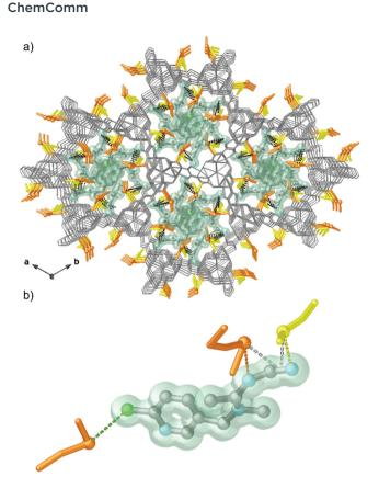
Fig. 9 (a) Perspective view, in the ab plane, of the porous structure of bioMOF Cu<sub>6</sub>SrMet/Mecys with acetamiprid molecules embedded. (b) Detailed view of the captured acetamiprid molecules emphasising the host-guest interactions with thioether groups from L-methionine and Smethyl-L-cysteine amino acids. Guest molecules are represented as green solid surfaces for the sake of clarity. This figure is adapted with permission from ref. 81, copyright ACS 2021.
