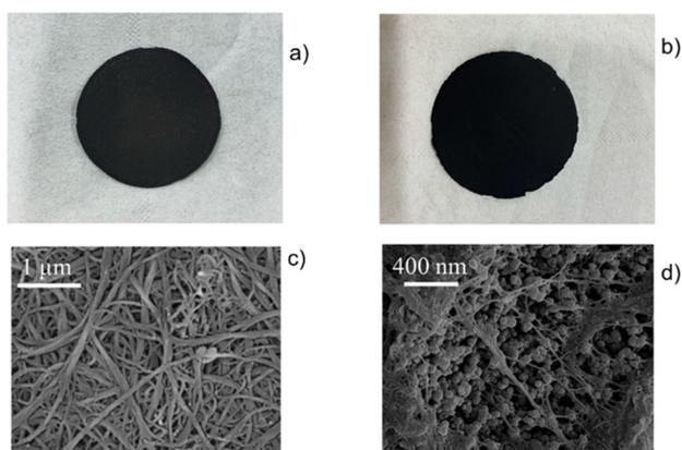
**Fig. 13** Photographs of neat SWCNT-BP (a) and bioMOF@SWCNT-BP obtained by integrating **Cu<sub>6</sub>SrThreo** and SWCNT-BP (b) circular membranes own an average diameter of  $41 \pm 1$  mm. SEM images of SWCNT-BP (c) and bioMOF@SWCNT-BP (d). This figure is reproduced with permission from ref. 78, copyright ACS 2022.
