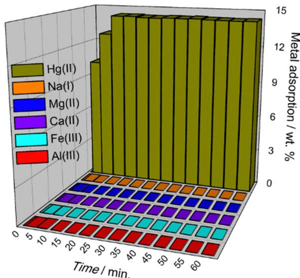
Fig. 5 Kinetic profile of the selective Hg(II) recovery by bioMOF **Cu<sub>6</sub>CaMet** represented as metal adsorption (wt%) vs. time in the presence of other interfering metal cations.
