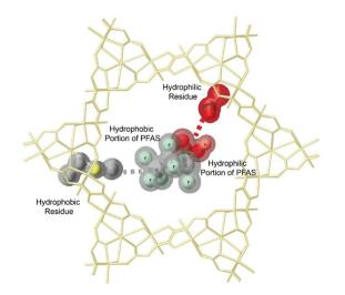
Fig. 14 Schematic representation of the capture mechanism suggested for MTV-bioMOFs towards PFAS
