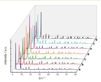
Fig. 2 (a) Calculated PXRD pattern profile of Cu<sub>6</sub>CaAla. Variable temperature XRD patterns of the activated phase of Cu<sub>6</sub>CaAla at 298 (b), 343 (c), 353 (d), and 370 K (e). PXRD pattern profiles of 1 after proton conduction measurements (f) and after 1 month immersed in a pH = 14 aqueous solution (g) at RT. This figure is reproduced with permission from ref. 66, copyright ACS 2016.
