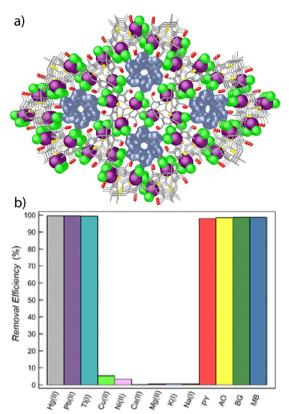
Fig. 11 (a) Details of crystal structure of MTV-bioMOF Cu<sub>6</sub>CaMet/Mecys after the simultaneous capture of HaCl2 and methylene blue. Mercury and chlorine atoms are represented by magenta and green spheres, respectively, whereas methylene blue molecules are represented as blue surfaces. (b) Maximum recovery (after 6 h) of both inorganic and organic contaminants. This figure is adapted with permission from ref. 83, copyright ACS 2019.
