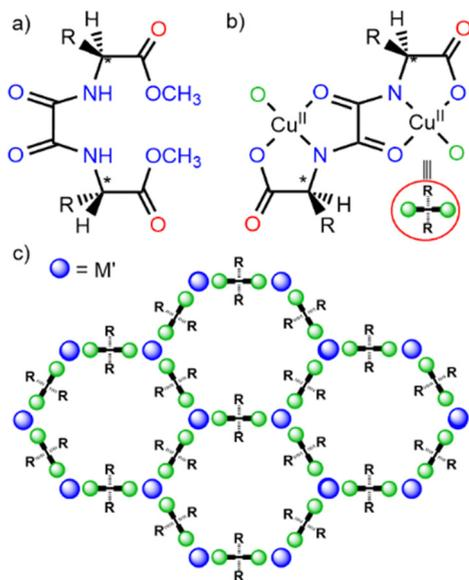
**Scheme 1** Chemical structures of the amino acid-based oxamidato ligands (a) and dicopper(II) precursor complexes (b), as well as a schematic representation of the bioMOF hexagonal network emphasizing the position of the amino acid residues (c). R represent the amino acid residues decorating the channels.
