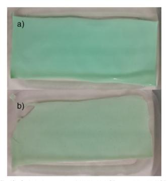
Fig. 12 Optical photographs of MMMs-bioMOFs containing bioMOFs  ${Ca^{II}Cu_{6}^{II}[(S,S)-methox]_{3}(OH)_{2}(H_{2}O)}\cdot 16H_{2}O$ (a) and  $\{Ca^{\parallel}Cu_{\varepsilon}^{\parallel}[(S,S)-$ Mecysmox]<sub>3</sub>(OH)<sub>2</sub>(H<sub>2</sub>O)}·16H<sub>2</sub>O (b). This figure is adapted with permission from ref. 77, copyright Wiley & Sons 2021.
