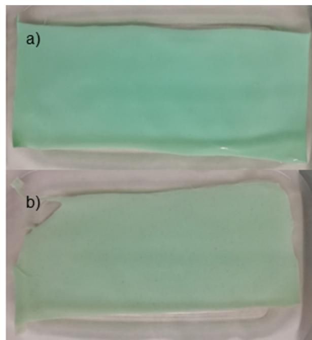
Fig. 12 Optical photographs of MMMs-bioMOFs containing bioMOFs  $\{\text{Ca}^{\text{II}}\text{Cu}_6^{\text{II}}[(\text{S,S})\text{-methox}]_3(\text{OH})_2(\text{H}_2\text{O})\}\cdot 16\text{H}_2\text{O}$  (a) and  $\{\text{Ca}^{\text{II}}\text{Cu}_6^{\text{II}}[(\text{S,S})\text{-Mecysmox}]_3(\text{OH})_2(\text{H}_2\text{O})\}\cdot 16\text{H}_2\text{O}$  (b). This figure is adapted with permission from ref. 77, copyright Wiley & Sons 2021.
