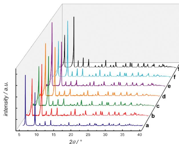
**Fig. 2** (a) Calculated PXR profile of **Cu<sub>6</sub>CaAla**. Variable temperature XRD patterns of the activated phase of **Cu<sub>6</sub>CaAla** at 298 (b), 343 (c), 353 (d), and 370 K (e). PXR pattern profiles of 1 after proton conduction measurements (f) and after 1 month immersed in a pH = 14 aqueous solution (g) at RT. This figure is reproduced with permission from ref. 66, copyright ACS 2016.
