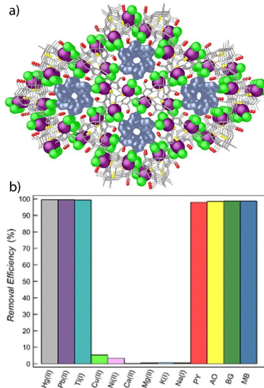
Fig. 11 (a) Details of crystal structure of MTV-bioMOF **Cu<sub>6</sub>CaMet/Mecys** after the simultaneous capture of HgCl<sub>2</sub> and methylene blue. Mercury and chlorine atoms are represented by magenta and green spheres, respectively, whereas methylene blue molecules are represented as blue surfaces. (b) Maximum recovery (after 6 h) of both inorganic and organic contaminants. This figure is adapted with permission from ref. 83, copyright ACS 2019.
