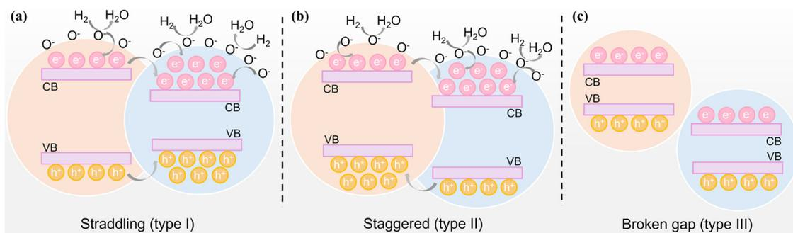
Fig. 8 Schematic of three types of heterojunctions. (a) Type of straddling. (b) Type of staggered. (c) Type of broken gap.
