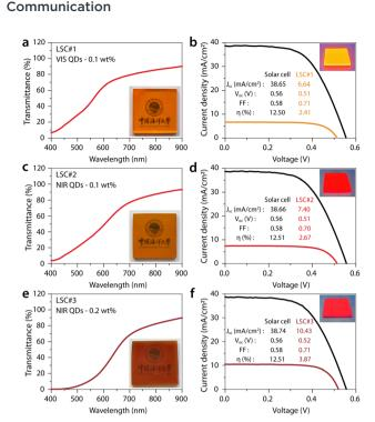
Fig. 4 (a), (c) and (e) Transmission spectra of LSCs with different types and concentrations of QDs. Insets show the planar LSCs under ambient light. (b) and (d) and (f) I-V curves of the as-prepared LSC prototypes (5  $\times$  5  $\times$  0.5 cm) and the coupled silicon cells. They were measured with a sunlight simulator under AM1.5 illumination. Insets show the digital images of LSCs under 365 nm UV light.
