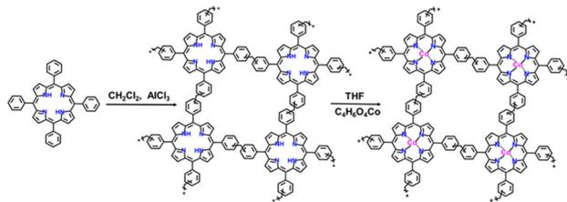
Fig. 1 Synthesis of a cobalt-tetraphenylporphyrin-based hyper cross-linked polymer.
