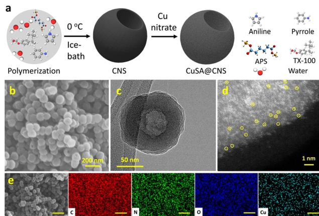
**Fig. 1** Microscopy and structural characterization of CuSA@CNS. (a) Schematics of fabrication processes. (b) SEM, (c) STEM, and (d) Cs-corrected HAADF-STEM images of CuSA@CNS catalysts. (e) HAADF-STEM image and the elemental distribution maps for C, N, O, and Cu of CuSA@CNS. Scale: 400 nm.
