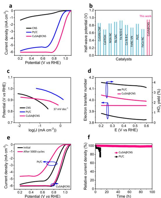
**Fig. 3** ORR electrochemical performances. (a) LSV profiles of CuSA@CNS associated with those of CNS and reference Pt/C catalysts. (b) Ragone plots of ORR half-wave potentials. (c) Tafel slopes. (d) The electron transfer number and peroxide yield. (e) ORR accelerated durability. (f) The  $i-t$  stability measurements.
