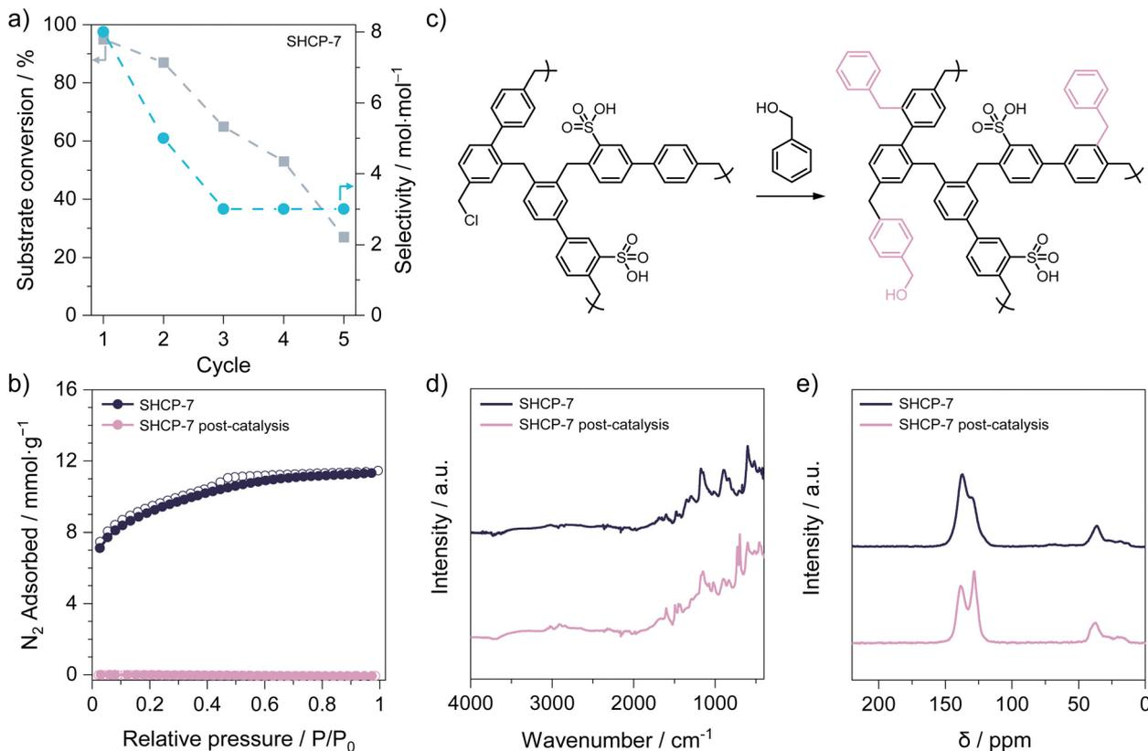
Fig. 2 (a) Catalytic efficiency of SHCP-7 across five cycles, showing benzyl alcohol conversion and ester/ether selectivity. (b) N<sub>2</sub> sorption–desorption isotherms of SHCP-7 (dark blue) before and after (pink) cycling, measured at  $-196$  °C. (c) Scheme of benzyl alcohol condensation onto an SHCP, the proposed cause of gradual catalytic decline. (d) FTIR spectra and (e) <sup>13</sup>C CP/MAS ssNMR of SHCP-7 before and after cycling.
