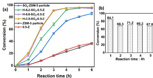
**Fig. 3** Conversion rate of oleic acid with methanol using sulfonated zeolite monoliths as catalysts. (a) The sulfonated monolith catalysts compared with ZSM-5 particles and the non-sulfonated zeolite monolith. (b) Reuse of the sulfonated monolith catalyst H-0.2-SO<sub>3</sub>-0.5-Z for five cycles. Reaction conditions: temperature 120 °C, catalyst loading: 5 wt%, molar ratio of methanol and oleic acid 10 : 1.
