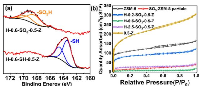
**Fig. 2** Characterization of ZSM-5 zeolite materials. (a) XPS spectrum of H-0.6- $\text{SO}_3\text{-0.5-Z}$  and H-0.6-SH-0.5-Z (b)  $\text{N}_2$  adsorption-desorption isotherms of ZSM-5 particles and monoliths.
