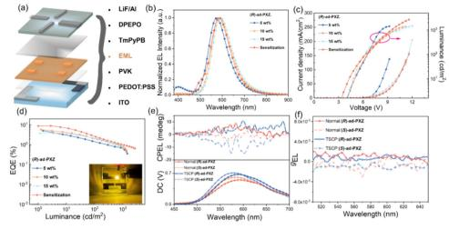
Fig. 4 (a) The structures of the solution-processable OLED materials; (b) normalized EL spectra of (R)-ad-PXZ; (c) current density-voltage-luminance (J-V-L) characteristics; (d) external quantum efficiency versus luminance (EQE-L) curves; (e) CPEL spectra and DC spectra of (R)-ad-PXZ/(S)-ad-PXZ; (f)  $q_{FI}$  spectra of (R)-ad-PXZ/(S)-ad-PXZ
