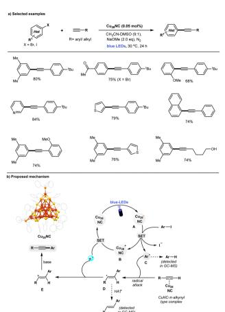
Fig. 3 Defects Cu<sub>28</sub> NC catalyzed Sonogashira C-C coupling reactions under photoinduced conditions
