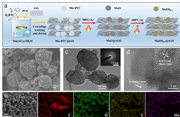
Fig. 1 (a) Scheme of synthetic process of  $\text{MnOS}_{0.3}@r\text{GO}$ . (b) SEM image, (c) TEM image and SAED image (inset), (d) HRTEM image with clear lattice fringes (inset), and (e) EDS and element mapping images of  $\text{MnOS}_{0.3}@r\text{GO}$ .
