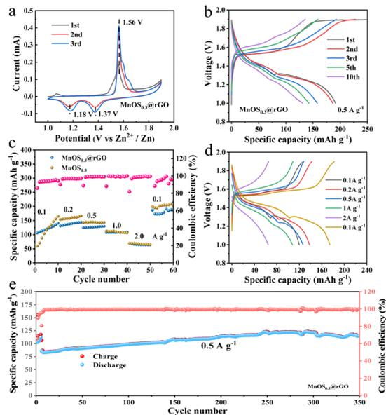
**Fig. 3** (a) CV curves of  $\text{MnOS}_{0.3}\text{@rGO}$  at a scanning rate of  $0.1 \text{ mV s}^{-1}$ ; (b) charging and discharging curves of different cycle number at a current density of  $0.5 \text{ A g}^{-1}$ ; (c) rate capabilities; (d) charge/discharge curves of  $\text{MnOS}_{0.3}\text{@rGO}$  at different current densities; and (e) cycling performance at  $0.5 \text{ A g}^{-1}$  for the  $\text{MnOS}_{0.3}\text{@rGO}$  electrodes.
