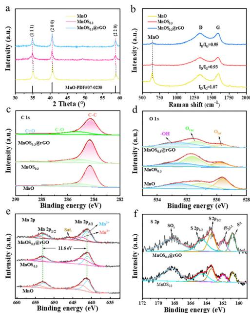
Fig. 2 (a) XRD patterns, (b) Raman spectra, (c) C 1s XPS spectra, (d) O 1s XPS spectra; (e) Mn 2p XPS spectra of MnO,  $\text{MnOS}_{0.3}$ , and  $\text{MnOS}_{0.3}@r\text{GO}$ ; and (f) S 2p XPS spectra  $\text{MnOS}_{0.3}$  and  $\text{MnOS}_{0.3}@r\text{GO}$ .
