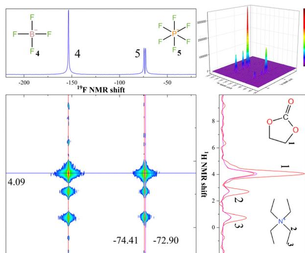
Fig. 6 <sup>1</sup>H–<sup>19</sup>F HOESY spectra for the 0.9 M TEABF<sub>4</sub> + 0.6 M TEAPF<sub>6</sub>-EC electrolyte solution.
