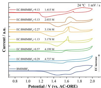
Fig. 1 Cyclic voltammograms of graphite electrodes in the electrolyte solutions of BMIMBF<sub>4</sub>-EC in the initial cycle.
