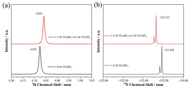
Fig. 7 (a)  $^1\text{H}$  and (b)  $^{19}\text{F}$  NMR spectra for the 1.5 M TEABF<sub>4</sub> + 0.3 M TEAPF<sub>6</sub>-EC and 1.8 M TEABF<sub>4</sub>-EC solutions.
