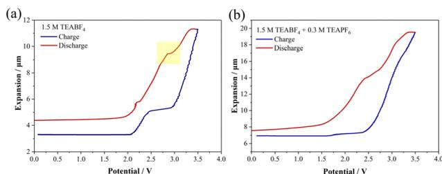
Fig. 5 ECD curves of graphite electrode in the (a) 1.5 M TEABF<sub>4</sub>-EC and (b) 1.5 M TEABF<sub>4</sub> + 0.3 M TEAPF<sub>6</sub>-EC electrolyte solution.
