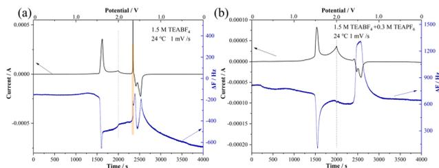
Fig. 4 CV-QCM curves of graphite electrode in the (a) 1.5 M TEABF<sub>4</sub>-EC and (b) 1.5 M TEABF<sub>4</sub> + 0.3 M TEAPF<sub>6</sub>-EC electrolyte solution.
