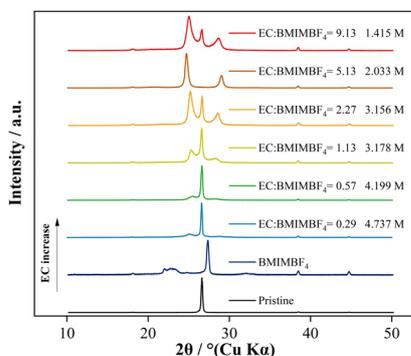
Fig. 2 *Ex situ* XRD patterns of graphite electrodes recovered from the AC/graphite cells charged to 3.5 V by utilizing the electrolyte of BMIMBF<sub>4</sub>-EC.
