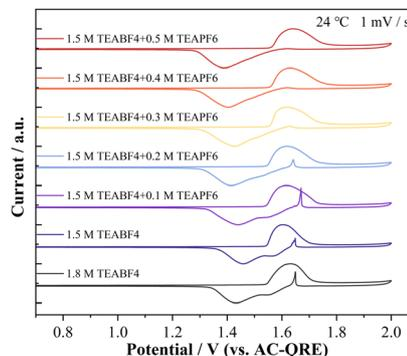
Fig. 3 Cyclic voltammograms of graphite electrodes in the electrolyte solutions of (TEABF<sub>4</sub> + TEAPF<sub>6</sub>)-EC in the initial cycle.
