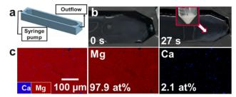
Fig. 3 Flow-gel device (a) schematics of the high-throughput prototype, (b) snapshots showing precipitate formation within 1 min, (c) EDS maps of precipitate obtained at a flow rate of 30 mL min<sup>-1</sup>.
