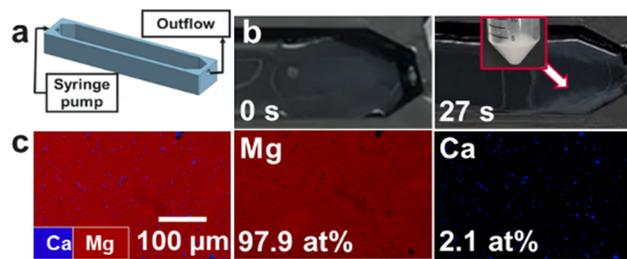
Fig. 3 Flow-gel device (a) schematics of the high-throughput prototype, (b) snapshots showing precipitate formation within 1 min, (c) EDS maps of precipitate obtained at a flow rate of  $30\text{ mL min}^{-1}$ .
