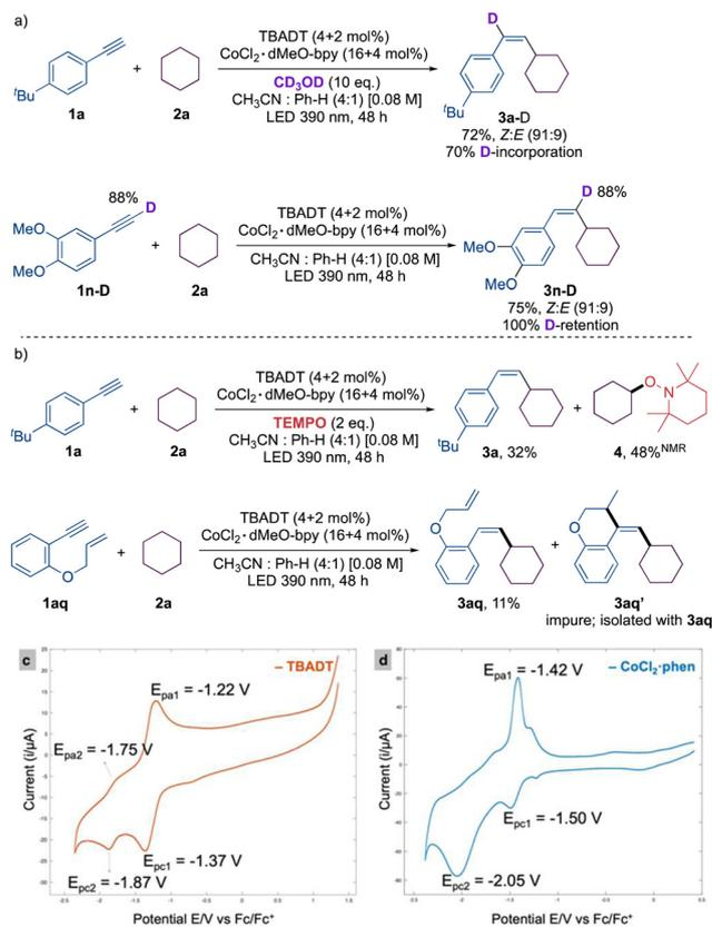
Scheme 2 (a) Deuterium labelling experiments, and (b) radical trap experiments. Cyclic voltammogram of (c) TBADT and (d) CoCl<sub>2</sub>·1,10-phenanthroline.
