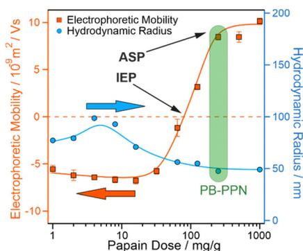
**Fig. 1** Electrophoretic mobility and hydrodynamic radius values in PB-PPN systems as a function of PPN dose. A PB concentration of 40 ppm and an ionic strength of 10 mM were maintained throughout the experiment. The chosen PPN dose of 250 mg g<sup>-1</sup> is marked with a green area (PB-PPN). The mg g<sup>-1</sup> unit refers to mg PPN per one gram of PB.
