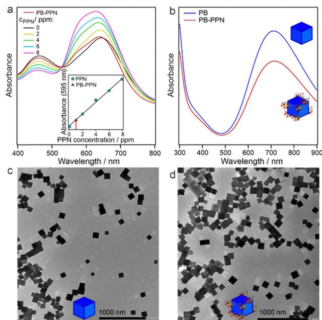
**Fig. 2** UV-Vis spectra recorded in the Bradford test with PPN dilution series and 40 ppm PB-PPN (a). The inset shows the absorbances of the series and PB-PPN at 595 nm as a function of free PPN concentration. UV-Vis spectra of PB and PB-PPN at 40 ppm concentration at pH 4 (b). TEM micrographs of PB nanocubes (c) and PB-PPN particles (d).
