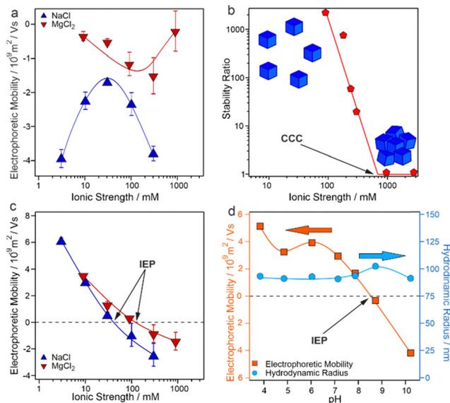
**Fig. 3** Electrophoretic mobility of PB as a function of ionic strength in NaCl and MgCl<sub>2</sub> solutions (a). Stability ratio of PB versus ionic strength in MgCl<sub>2</sub> electrolyte (b). Electrophoretic mobility of PB-PPN as a function of the ionic strength in NaCl and MgCl<sub>2</sub> (c). The pH-dependence of electrophoretic mobility and hydrodynamic radius of PB-PPN (d). Particle concentrations were always maintained at 40 ppm.
