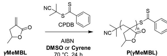
**Scheme 1** Reaction scheme for the RAFT solution polymerisation of  $\gamma$ MeMBL with either DMSO or Cyrene as the solvent at 70 °C.
