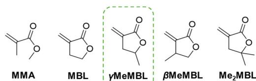
Fig. 1 Chemical structures of MMA and the family of 5-membered  $\alpha$ -methylene- $\gamma$ -butyrolactone monomers; MBL,  $\gamma$ MeMBL,  $\beta$ MeMBL and Me<sub>2</sub>MBL.
