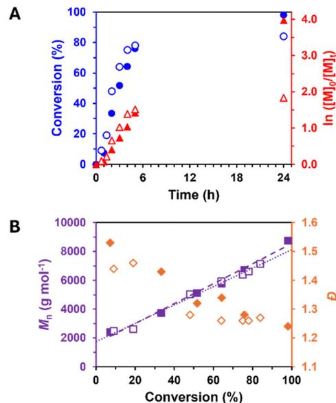
Fig. 3 Kinetic evaluations of the synthesis of  $P(\gamma$ MeMBL) $_{100}$  by RAFT solution polymerisation of  $\gamma$ MeMBL at 70 °C in DMSO (closed symbols) and Cyrene (open symbols); (A) conversion (blue circles) and the rate of polymerisation (red triangles) *versus* time, and (B)  $M_n$  (purple squares) and  $D$  (orange diamonds) *versus* conversion. The dashed and dotted lines show the linear increase in  $M_n$  in DMSO and Cyrene, respectively.
