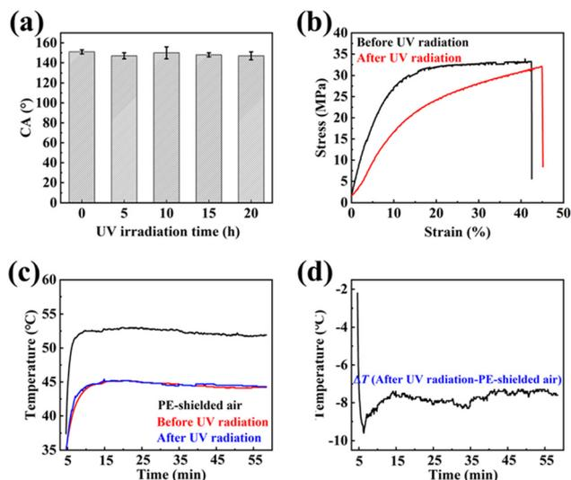
Fig. 4 (a) Contact angle of PVDF/SiO<sub>2</sub> composite films at different UV aging times; (b) stress–strain curves of PVDF/SiO<sub>2</sub> composite films before and after UV radiation (radiation for 20 h); (c) real-time temperature profiles of PVDF/SiO<sub>2</sub> composite films under a xenon lamp before and after UV radiation; (d) average temperature drop ( $\Delta T$ ) of the PVDF/SiO<sub>2</sub> composite film after UV radiation and PE covered air.
