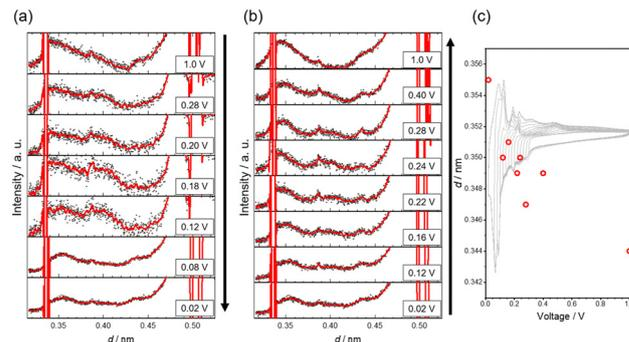
**Fig. 4** *In situ* XRD patterns for a SE-cell during (a) charging and (b) discharging. Weaker intensity at 1.00–0.12 V at the charging process is due to beam adjustment to enhance the signal-to-noise ratio. The abscissa is the value of  $2\theta$  converted to  $d$ -values based on the X-ray wavelength (0.0827 nm). (c) The  $d$ -values for voltage during the discharge process.
