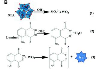
Fig. 3 (A) The relationship between CL intensities and time for the luminol/H<sub>2</sub>O<sub>2</sub> system and luminol/STA system [luminol]: 10 μM; [STA]: 2 mM;  $[H_2O_2]$ : 2 mM; pH: 12.0; PMT voltage: -950 V. (B) The CL mechanism of the luminol/STA system. Reprinted with permission from ref. 42, Copyright 2020 Royal Society of Chemistry.
