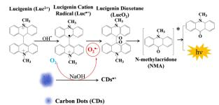
Scheme 2 Schematic representation of the lucigenin-CD CL system in NaOH solution. Reprinted with permission from ref. 52, Copyright 2019 Springer Nature.
