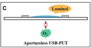
Fig. 15 Comparison between an apertureless USB-PUT and a USB-PUT with microtapered apertures. (A) Effect of H<sub>2</sub>O<sub>2</sub> concentration. (B) Principle of the USB-PUT with microtapered apertures. (C) Apertureless USB-PUT.  $[H_2O_2]$ : 0.5-1000  $\mu$ M, [luminol]: 100  $\mu$ M in pH 12 CBS buffer. Reprinted with permission from ref. 66, Copyright 2021 American Chemical Society
