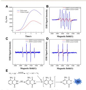
**Fig. 12** (A) CL kinetic curves of the luminol/FeOOH system in the absence and presence of oxygen. ESR spectra of adducts. (B) DMPO- $O_2^{\bullet-}$  (C) DMPO-OH $^{\bullet}$  and (D) TEMP- $^1O_2$  in the luminol/FeOOH CL system. (D) Mechanism of the luminol/FeOOH CL system. (E) The mechanism of the luminol/FeOOH system. [Luminol]: 100 μM; [FeOOH]: 25 μg mL $^{-1}$ ; [UA]: 5 μM; [pH]: 10.0. Reprinted with permission from ref. 63, Copyright 2023 American Chemical Society.
