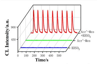
Fig. 7 CL intensity-time curves of KHSO<sub>5</sub>, Acr<sup>+</sup>-Mes, and Acr<sup>+</sup>-Mes/  $KHSO_5$  systems. [Acr<sup>+</sup>-Mes]: 0.1 mM; [KHSO<sub>5</sub>]: 2 mM; [PBS]: 0.1 M, pH = 7; PMT voltage: -900 V. Reprinted with permission from ref. 15, Copyright 2023 American Chemical Society.
