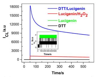
Fig. 5 CL intensity versus time profiles for the systems of lucigenin/DTT, lucigenin/H<sub>2</sub>O<sub>2</sub>, lucigenin, and DTT. Inset: enlarged CL emissions of DTT and lucigenin. [lucigenin]: 0.1 mM; [DTT]: 1.0 mM; [H<sub>2</sub>O<sub>2</sub>] 1.0 mM; 0.1 M PBS (pH 11); PMT voltage: -750 V. Reprinted with permission from ref. 45, Copyright 2022 American Chemical Society
