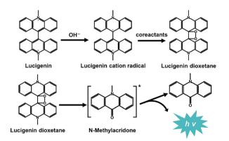
Scheme 1 Mechanism of lucigenin-based CL systems.
