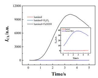
Fig. 11 The CL intensity—time curves of luminol, luminol/ $H_2O_2$  and luminol/FeOOH systems. [Luminol]: 100  $\mu$ M; [FeOOH]: 25  $\mu$ g mL<sup>-1</sup>; [ $H_2O_2$ ]: 1  $\mu$ M; [pH]: 10.0. Reprinted with permission from ref. 63, Copyright 2023, American Chemical Society.
