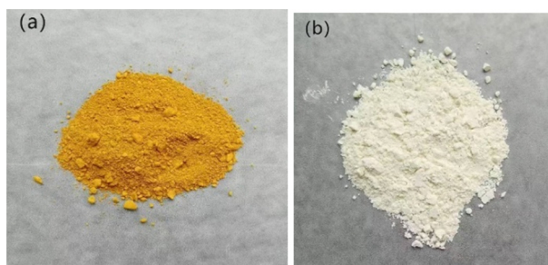
Fig. 1 Optical photographs of the high-pressure hydrolyzed precipitates (a), and the synthesized \text{FePO}_4 \cdot 2\text{H}_2\text{O} samples (b).
