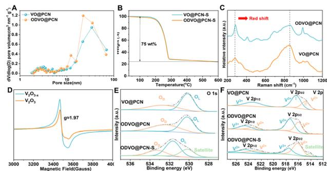
**Fig. 2** (A) Pore size distribution of ODVO@PCN and VO@PCN; (B) thermogravimetric analysis (TGA) curves of ODVO@PCN-S and VO@PCN-S nanocomposites; (C) characteristic Raman spectra of the ODVO@PCN and VO@PCN nanocomposites; (D) EPR spectra of the as-synthesized ODVO@PCN and VO@PCN nanocomposites; high-resolution spectra of (E) O 1s and (F) V 2p of the ODVO@PCN, ODVO@PCN-S and VO@PCN nanocomposites.
