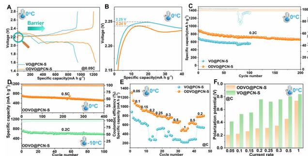
Fig. 4 (A) Initial charge–discharge profiles of the ODVO@PCN-S and VO@PCN-S cathodes at 0.05C; (B) comparison of the corresponding decomposition potential of  $Li_2S$  on the two cathodes; (C) cycle performance of the cathodes at 0.2C; (D) cycle performance of the ODVO@PCN-S cathodes at 0.5C (0 °C) and at 0.2C (–10 °C), respectively; (E) rate performance of the cathodes; (F) comparison of the overpotential at rates varying from 0.05 to 1C under low temperature.
