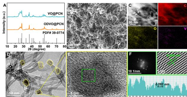
**Fig. 1** (A) XRD curves of VO@PCN and ODVO@PCN nanocomposites; (B) SEM image and (C) STEM image, and corresponding EDX elemental mappings; (D) TEM image, (E) HRTEM image, and (F) FFT and IFFT images of the highlighted area of the ODVO@PCN nanocomposite.
